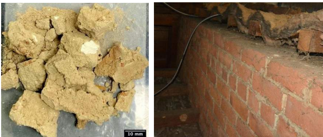
Figure B9. Mortar sample FM-01 and location from south elevation brick wall exposed in attic.
