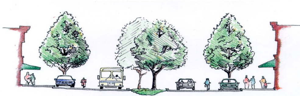
Figure LU-11, Pedestrian Oriented Roadway Section
