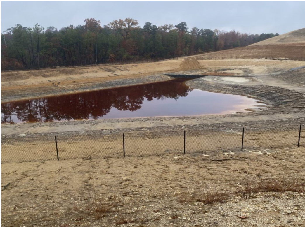
Figure 5. Exposure of acid sulfate soil (ASS) materials in a deep stormwater pond excavation in Miocene age Coastal Plain sediments in the Fredericksburg area. The darker gray sulfidic materials are reduced (anaerobic) and then oxidize to form sulfuric acid and very low pH (< 3.5) and metal enrichment (Al, Fe and Mn) in soil and receiving waters. Remediation of these materials requires very heavy lime applications (> 15-50 tons ag lime per acre six inches). Note: This site is not from the area depicted in Figures 2 and 3 above, but these materials commonly occur at depth throughout the Coastal Plain, eastern Piedmont, and certain other Virginia locales.
