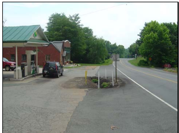
The existing access management of Rt. 15 should be improved with a coordinated plan of curb and gutter, clear driveway and pedestrian zones, and other devices.
