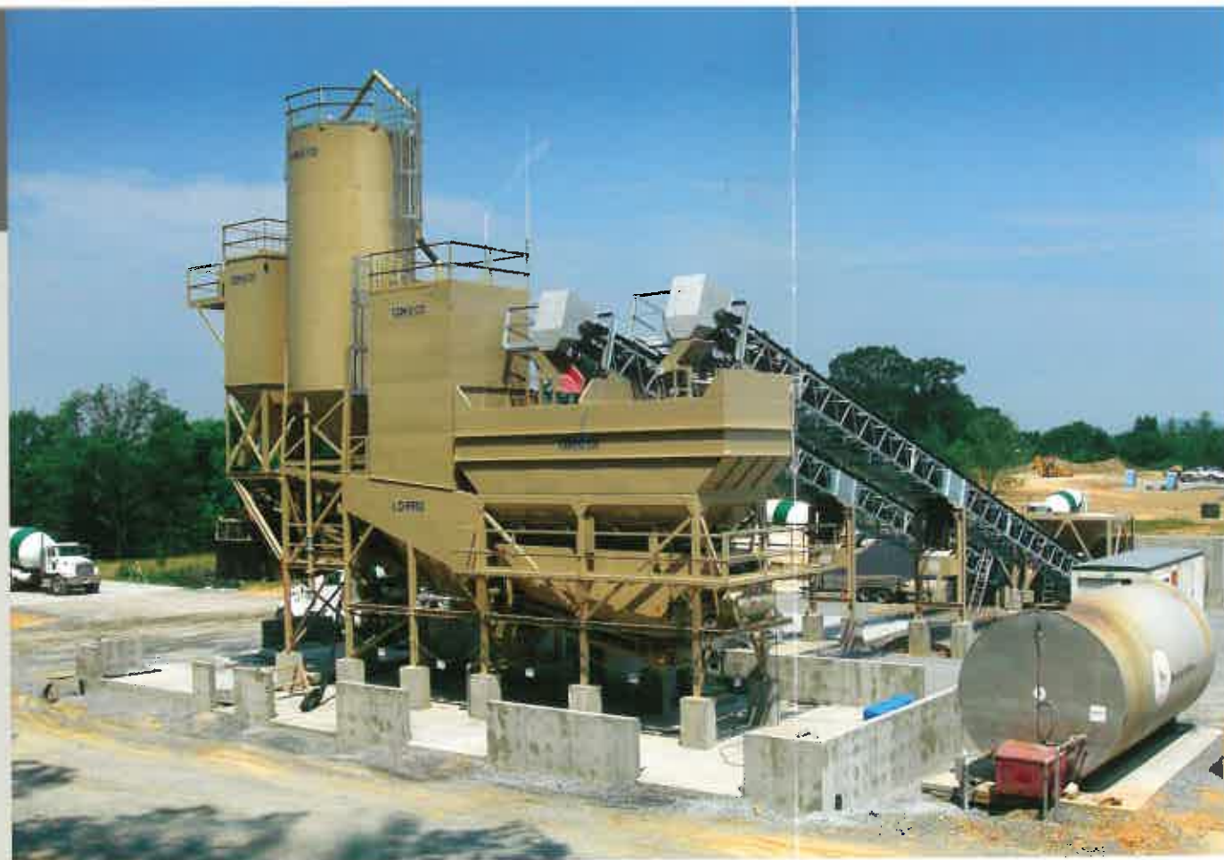
Wilson's LO-PRO 12 features two conveyors charging four aggregate compartments.
