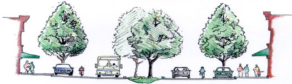
Figure LU-11, Pedestrian Oriented Roadway Section
