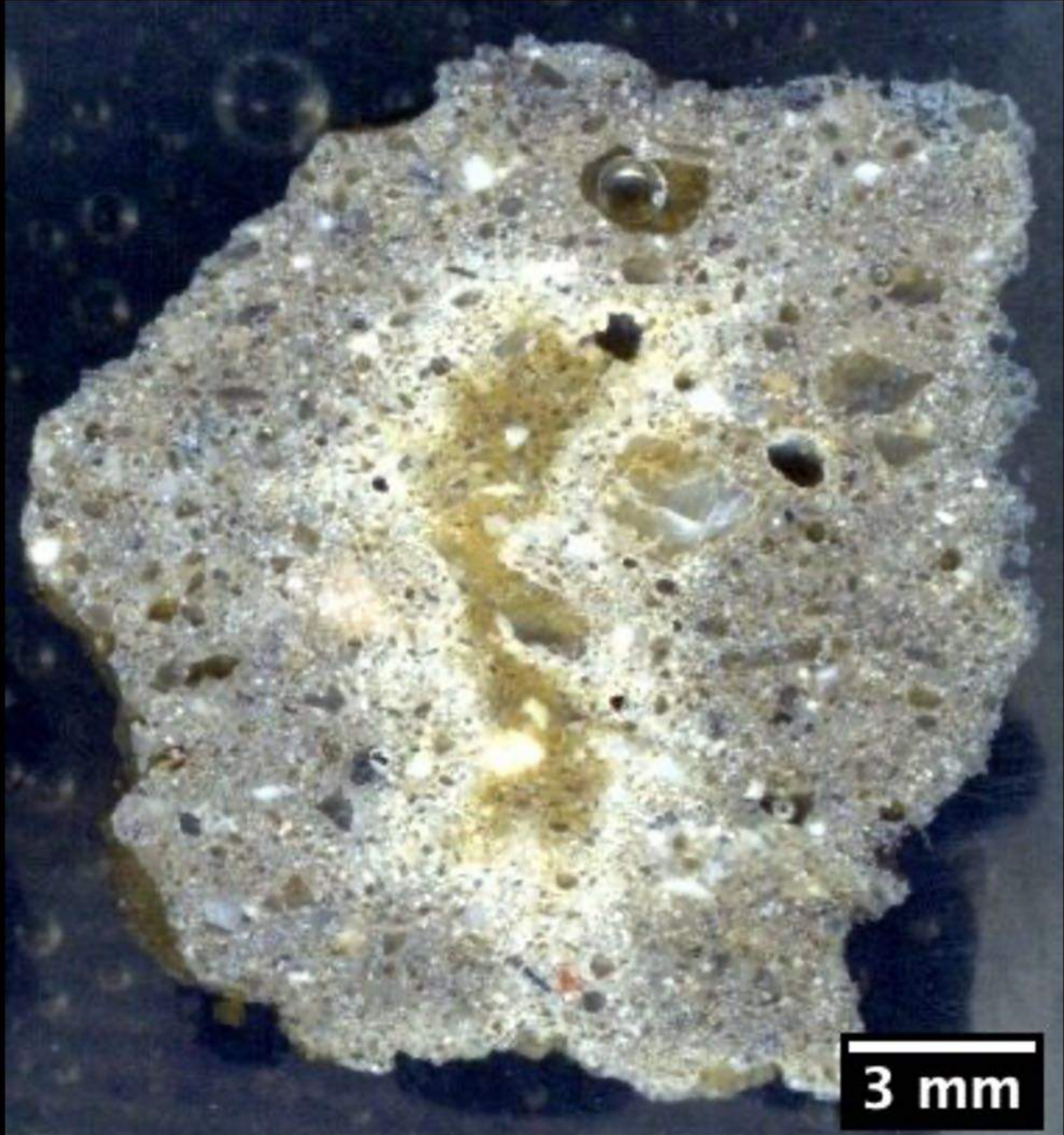
Figure 6: Clear epoxy-impregnated lapped cross section of a mortar fragment showing the size, shape, angularity, gradation, and distribution of sand particles, and interstitial paste fraction. The color variation from lighter gray core to darker gray rim is due to incomplete depth of encapsulation of clear epoxy and does not necessarily indicate true color tones of mortar.
