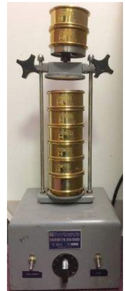
Fig. A1: Gilson mini sieve shaker used for sieve analysis of sand extract from mortar after acid digestion.
