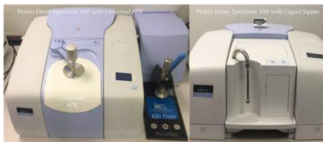
Fig. A10: Perkin Elmer Spectrum 100 FT-IR unit with Universal ATR attachment for examinations of coatings on mortars.
