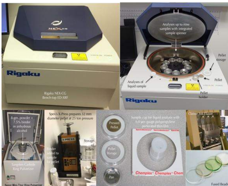
Fig. A8: Rigaku NEX-CG in CMC, which can perform analyses of 9 pressed pellet or fused bead of sample. Samples are prepared either as pressed pellet (usually the one already prepared for XRD) or can also accommodate fused bead with proper calibration of standard beads
