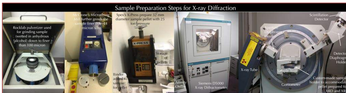
Fig. A7: Siemens D5000 X-ray diffractometer and MDI Jade search/match software used for determination of mineralogical composition of mortar. Left to right: Rocklab pulverizer for initial grinding of sample with anhydrous
