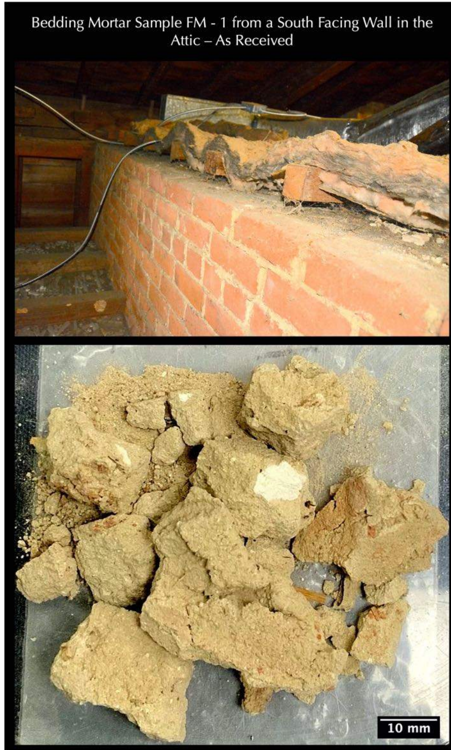
Figure 2: Location of the bed joint (top photo) from where the tan-colored fragments of mortar sample (bottom photo) was collected.
